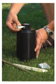
5. Install protective tip cap horizontally through plastic sleeve into anchor to lock the two together.
